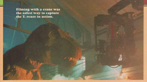
in refining their control systems so that the pair could perform in tandem. "What we ended up with was much heavier robots [9 tons each, as compared to *Jurassic Park*'s 9,000-pound lightweight] that were able to move faster and be more violent and stronger and, at the same time, could stop on a dime."
